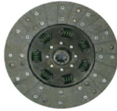
STP-1201 Clutch Plate DI (11") N/A Facing
