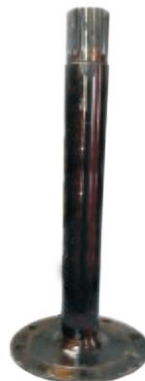
↑STP-5675 Rear Axle 13T Big Plate
