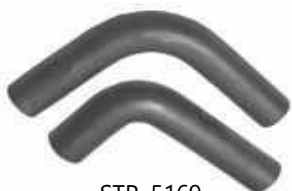
STP-5169 Hose Pipe Set 3Cyl DI [EPDM]
